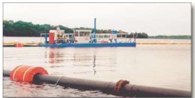
Manufactured by Ellicott Int'l., the MC-2000 was ideal for the BAAP project as it is transportable on one truck for easy mobilization to this remote location, and is efficient in lakes, bays, and rivers.
