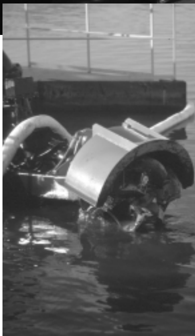
Shielded cutterhead of hydraulic dredge
